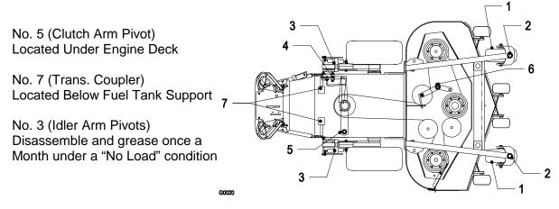
c) Lubricate pivot points with a spray penetrating lubricant as directed below.
